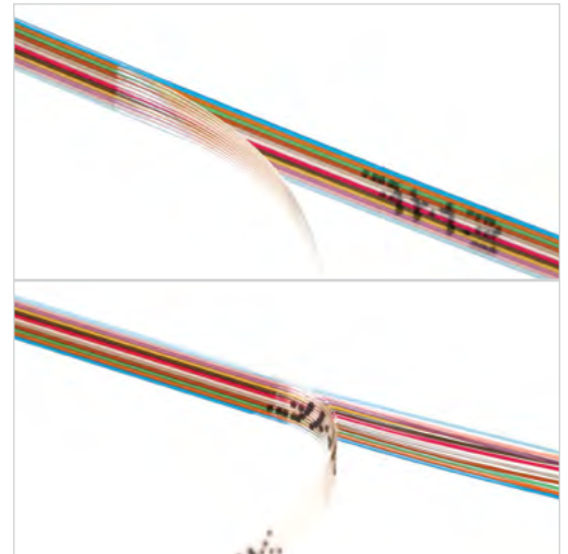
The ribbon matrix peels cleanly from both sides of the fiber.
