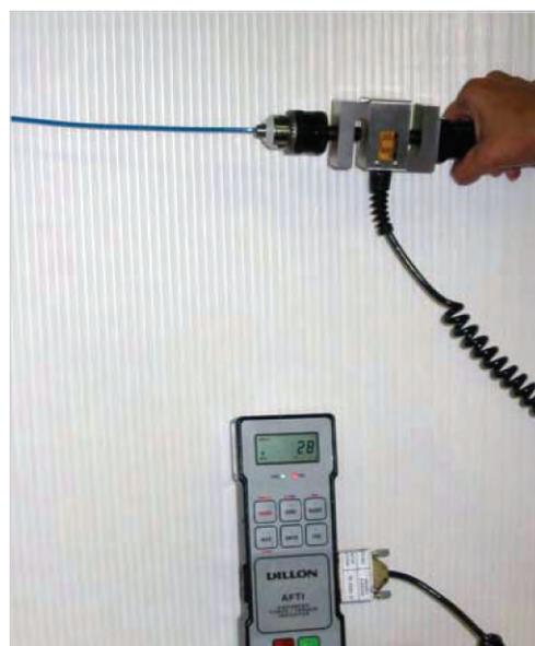
Figure 3: Removal Force Test
