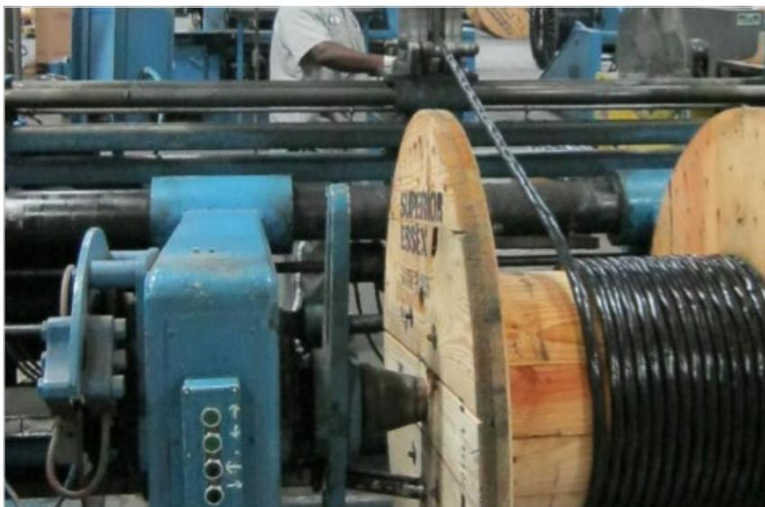
*Picture of cable being re-spooled from large reel to smaller reel*
